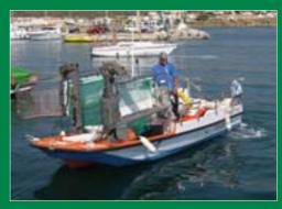
FCC uses 59 Marnett boats designed specifically for collecting floating and semi-submerged debris, seaweed and jellyfish in bathing areas.
