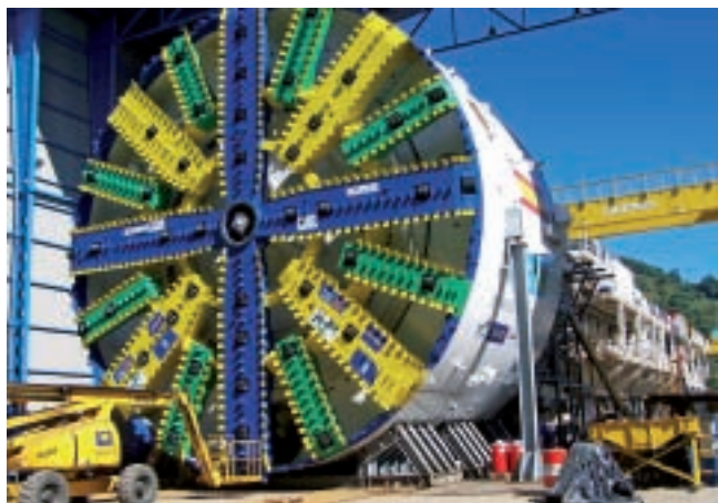
"Tizona", one of FCC's tunnel boring machines
