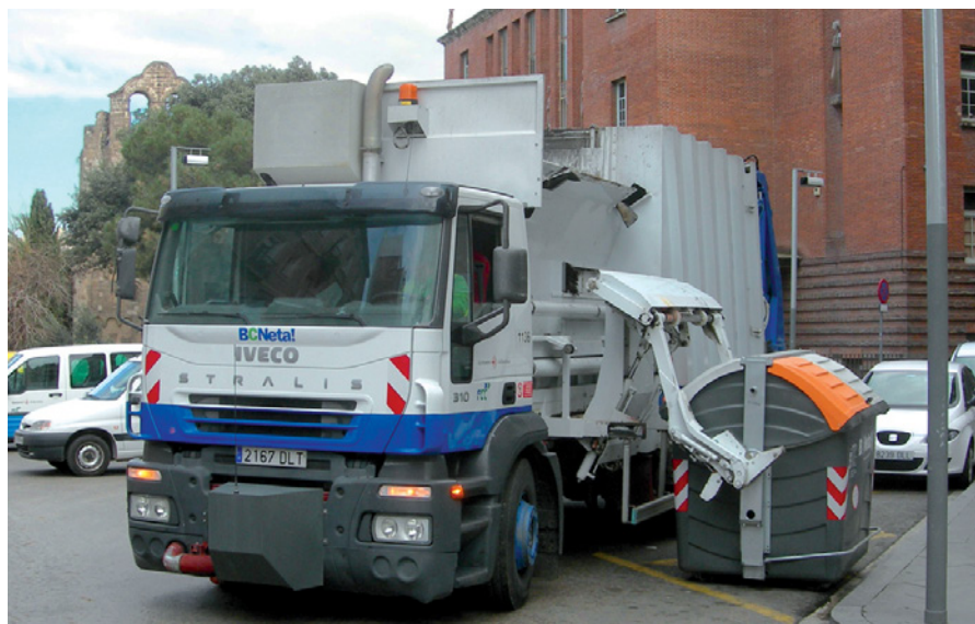
Solid urban waste collection service. Side loading vehicle. Barcelona
