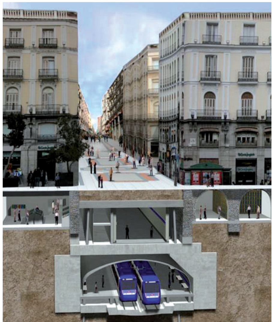
Extension of platforms and new entrance hallway for Sol station, Madrid metro line 3
